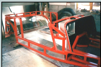
Painted chassis and aluminium inner bodywork in place
