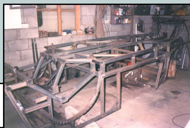
Substantial 2x2 box section chassis
